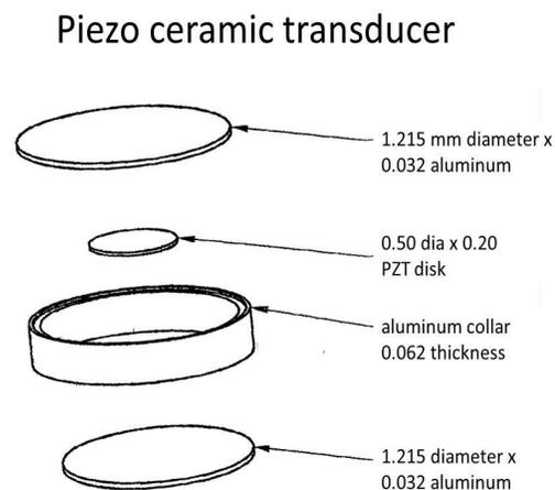
**Figure 1.** Components and dimensions of the prototype piezo ceramic transducer.
